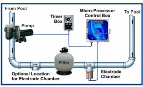
Basically, the current causes some of the outermost atoms of the electrodes to lose an electron, thus becoming positive ions. While the water is running through the chamber, many of these ions are swept away before they can reach the other side of the electrodes. As a result, the mineral ions are dispersed into the body of water that is being purified.
