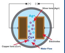
When the "used" mineral ions are removed, the microprocessor control box is always producing new mineral ions to continuously sanitize the water.
